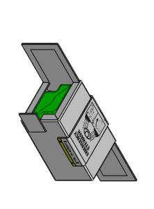
STEP 3: WRAP THE JACKET UP AND OVER THE 7501 TANK AND ATTACH THE BOTTOM VELCRO CLOSURES.
