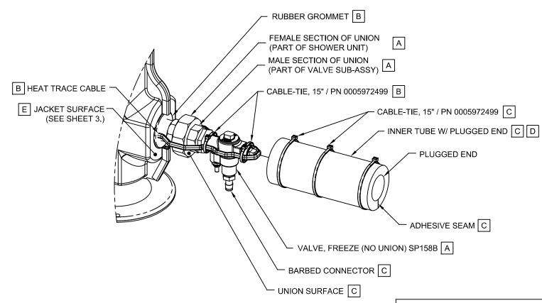
SP158B VALVE SHOWN CONNECTED TO BOTTOM UNION FOR REFERENCE ONLY. VALVE CAN BE INSTALLED AT TOP OR BOTTOM.
